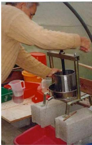
This pressing operation effects a more efficient separation of the residual culture medium than washing the biomass. Washing with fresh water may cause rupture of the cell wall of the spirulina due to osmotic shock, leading to loss of valuable products; it may also introduce germs contained in the wash water.
