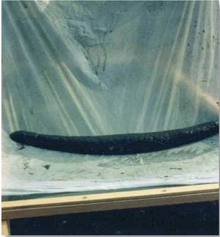
Filtration is done on a 30  $\mu$  mesh cloth. When most of the water has filtered through, the biomass will agglomerate into a "ball" under motion of the filtering cloth, leaving the cloth clean (this desirable condition happens when the biomass is richer in spiralled forms and the culture medium is clean). At this stage the biomass contains 10% dry matter and it has a soft consistency; it will not stick to plastic materials but glide on it.
