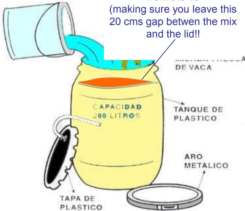
**Step 6.** Put the lid on, arm the iron ring around it secure it and hang a plastic bottle full of water from it..
