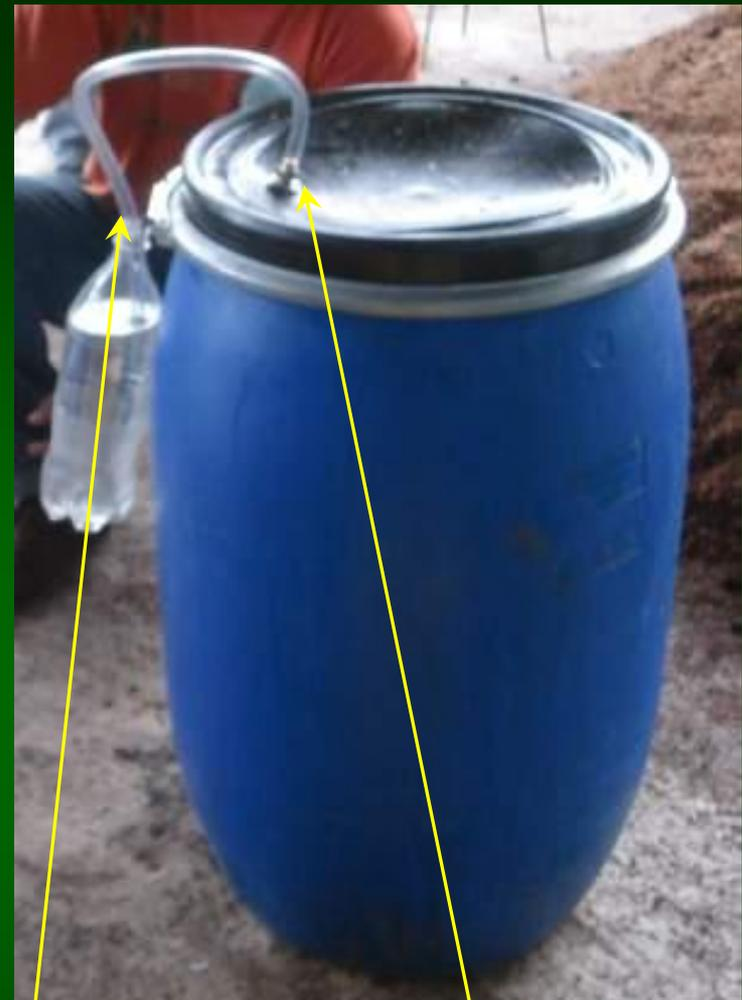
Insert one end of a 1/2" plastic hose in coupling and tighten it with a clamp.
