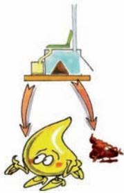
Urine diverting toilets do not mix urine and faeces by using a separating toilet seat. Urine is collected and stored in a reservoir. Faeces are collected underneath the toilet must be directly covered by dry materials such as saw dust, soil or ashes or a mixture of those, and stored for 2 years.
